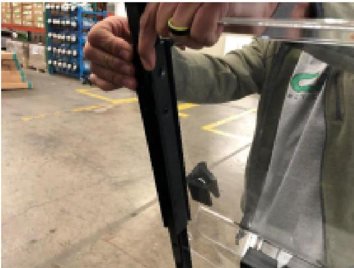
Perform this task on both sides. Once both sides have been released from the roof supports, you can pull the windshield off. If replacing the windshield, you will need to remove the black plastic retainers and reuse them on the new windshield.
